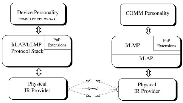
The above diagram illustrates the software stack on a typical IrDA approved PnP compatible device. The stack pictured on the left portrays a PnP ready OS and the layers required to support a
